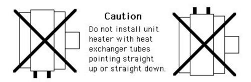
The heat exchanger tube in the upper most position should be connected to the return water line of the boiler system. Water lines should also include a air bleeder at or near the unit heater at the highest point of the lines. This will allow for proper removal of air from heat exchanger and ensure maximum unit heater performance. For the water and air specifications for this unit please refer to the dimensions and specification page of these instructions.
