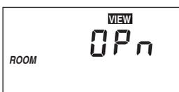
The control is no longer able to read the indoor sensor due to an open circuit. The control will continue to operate as if there was nothing connected to the indoor sensor input. Locate and repair the problem as described in the Data Brochure D 074. If the indoor sensor was deliberately removed, the control must be powered down, and then powered back up. To clear the error message from the control after the sensor has been repaired, press the **Item** button.
