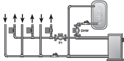
To prevent high temperature water from being introduced into the heating system, the boiler pump P1 must be turned off during a call for DHW. To do this, the DHW device must be a DHW pump (DIP switch = *DHW Pump*), DHW priority must be selected (DIP switch = *DHW Priority*), and BOIL MIN must be set to OFF.
