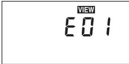
The control was unable to read a piece of information from its EEPROM. This error can be caused by a noisy power source. The control will load the factory defaults and stop operation until all the settings are verified.
