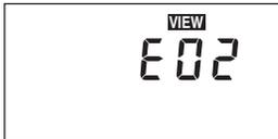
This error is caused by an illegal DHW DIP switch setting. When *DHW Priority* and *DHW Valve* are selected in the DIP switch settings, the control will flash the error message. In this case, the control will operate as if the *DHW Priority / Off* DIP switch is set to *Off*. To clear the error message from the control, set the *DHW Priority / Off* DIP switch to *Off* and press the **Item** button.
