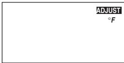
Press and release the **Item** button to advance to the units adjustment. Use the ▲ or ▼ button to set the scale to °F or °C.
