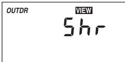
The control is no longer able to read the outdoor sensor due to a short circuit. In this case the control assumes an outdoor temperature of 32°F (0°C) and continues operation. Locate and repair the problem as described in the Data Brochure D 070. To clear the error message from the control after the sensor has been repaired, press the **Item** button.
