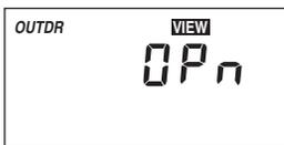
The control is no longer able to read the outdoor sensor due to an open circuit. In this case the control assumes an outdoor temperature of 32°F (0°C) and continues operation. Locate and repair the problem as described in the Data Brochure D 070. To clear the error message from the control after the sensor has been repaired, press the **Item** button.
