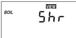
The control is no longer able to read the boiler sensor due to a short circuit. In this case the control does not operate the *Boiler* contact. Locate and repair the problem as described in the Data Brochure D 070. To clear the error message from the control after the sensor has been repaired, press the **Item** button.
