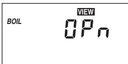
The control is no longer able to read the boiler sensor due to an open circuit. In this case the control does not operate the *Boiler* contact. Locate and repair the problem as described in the Data Brochure D 070. To clear the error message from the control after the sensor has been repaired, press the **Item** button.
