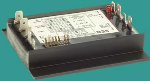
The **D35** pre-calibrated electronic controller is Thermolec's most flexible controller with four different input options on a single board. Jumper configurations are clearly indicated on the label and may be changed at any time. Control signals supported are Thermistor for Thermolec's RT, DT or RADS, 0-135 Ohms, 4-20 mA and 0 - 10 VDC. Since the D35 is not compatible with our Air Flow Sensor it is recommended to be used with a PDS (Pressure Differential Switch) instead.
